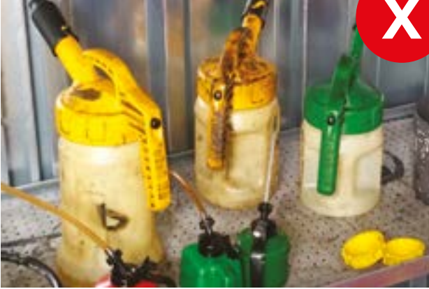
Unlabelled oil containers – these could easily lead to the wrong oil being used
